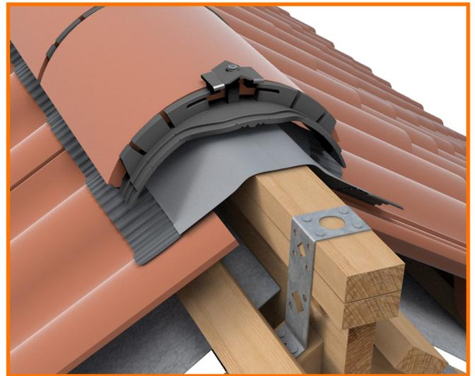
Fig 6. Fix ridge tile – 3D View.
