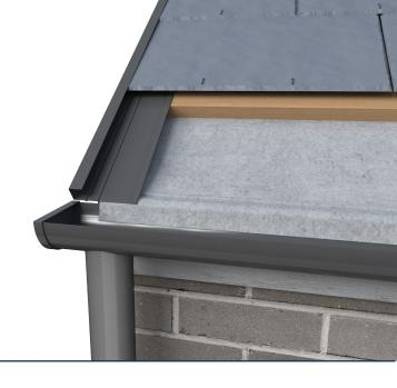
The Kytun™ Slate Dry Verge System Type 2 System secures slate applications on gable ends permanently protecting the verge from the elements especially wind uplift and rain.
