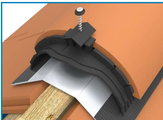
Fig 7. Fix roof tile. – 3D View.
